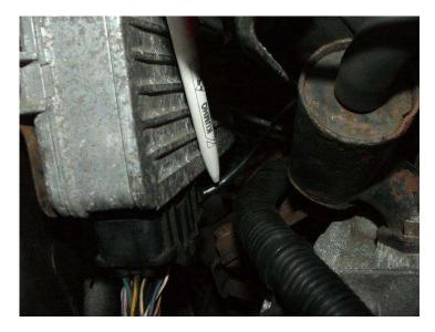
Other locations of air leaks are the breather system hoses and the evaperative emissions control system. Check all rubber hoses are in good condition, no cracks or splits. The main breather hoses to check are the ones supplying the purge valve and the charcoal canister. They usualy leak at the purge valve shown here.
