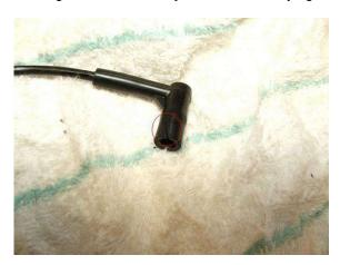
The main one that seems to cause a problem is the one on the end of the short capilary **identified with white**, from the back of the inlet manifold to the fuel trap. Located on this port on the back of the inlet manifold, again identified with white.
