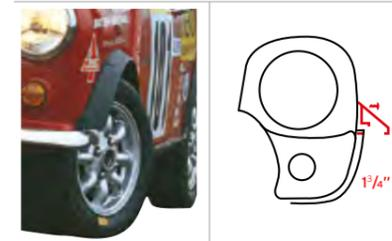
**Mini Special Arches.** Includes sill trim moulding between arches. This arch kit sticks out 1 3/4" when body line (wheel arch and moulding seam) are kept original. Originally fitted to Innocenti Minis and became standard equipment on all Minis from 1984. Screws are visible and rear arch extends beyond bumper seam line. These black plastic arches were originally known as Mini Special Arches GAW117
