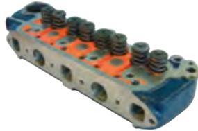
Unleaded with manganese bronze guides and race spec EN21 4N stainless steel heat treated valves to eradicate wear. £150 refundable surcharge (if head is in a condition suitable for reconditioning) unless stated otherwise
