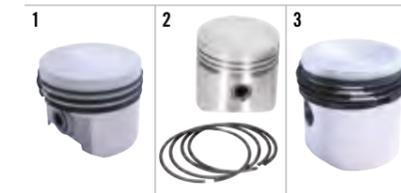
1. **998cc flat top piston with press fit gudgeon pins.** Low drag slipper pistons as fitted by Rover (TAM2052) in the last Minis and Metros. So reliable they have been used in race engines.
