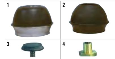
1 This shaped cone has a progressive balanced spring rate and when fitted initially sits higher than the standard original cones, HILOs will be required. Racers favourite Mini Spares product.
