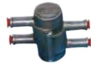
The Mocal oil control thermostat is designed to prevent flow of engine oil until it has reached correct working temperature of about 80°C. Prolonged use of engine oil where it cannot reach its correct working temperature can cause sludge and crank case dilution, leading to excessive wear in crank bearings and cylinder bores. Fits into any convenient place where pipes can be cut and oil pipes run parallel.
