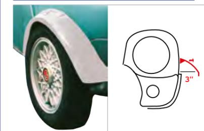
This arch kit sticks out 3" and is used when body line is cut away or retained. Originally made as Group 5 Race arch where no body modifications were required, it has become a cheap 'Jack of all Trades' especially when large odd size wheels are used. Rear arches stop at bumper seam line. Widest part at front approximately 5". White only MS128
