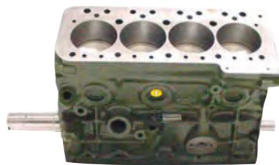
1. **Half engine.** Built up with oil pump, lightened cam followers, EVOLUTION001 camshaft as it gives a broad range of torque and power for fast road use with good acceptable economy and emission readings. Modified front plate to accept new duplex kit and dialed in with camshaft and distributor drive, so you will require an A Plus distributor. Your timing cover may require modifying to fit duplex or a new one can be supplied. £25.00 extra.
