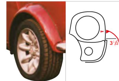
1 The last Rover arches, as fitted to the Sportspack Mini from 1997. Moulded rubber and stick out 3 1/2". The body line has to be cut away to fit. Finished in correct rubber primer.
