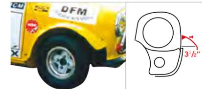
This arch kit sticks out a nominal 3 1/2" and more when positioned at the angle most racers use as shown. 5 1/2" wide at very front. Definitely only for cars with body line modifications and fairly inexpensive to replace. Rear arches stop at bumper seam line. White only MS128W
