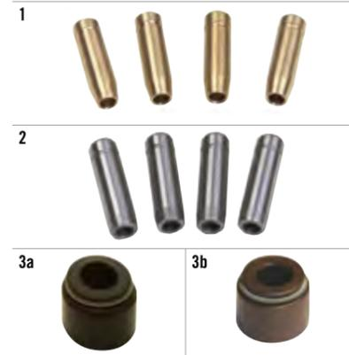
Although Silicon bronze valve guides were used for their extremely good wear values they were very hard and not user friendly when fitting. We have introduced the Manganese bronze guides which have good cutting properties and good wear characteristics and are original equipment on Porsche and Mercedes.
