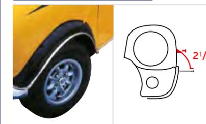
This arch kit sticks out 2 1/2", including lip, when body lines (wheel arch and moulding lip) are kept original. Screws are visible and plastic wheel arch moulding can be retained. Rear arch stops at bumper seam line. These are original ST works car copies. Black C-STN71
