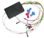
**Dash illumination & lights-on chime.** This upgrade will enable you to illuminate your dash switches to save you fumbling in the dark. The kit also adds a lights-on chime to avoid leaving your lights on and draining the battery **MSSK2007**
