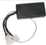
**This wiper delay conversion kit will allow normal fast and slow wiper operation,** but if you operate the 'flick-wipe' twice in succession it will 'learn' the delay between each flick and then allow intermittent wipes using this time delay.
