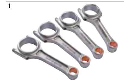
1. **Set of forged steel rods standard fitment 5.75" long** 1.625" journal size with 20.66mm standard gudgeon pin C-AEG624
