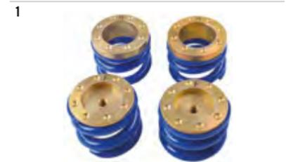
1 Softer cones in different shapes have proven to give a more comfortable ride but at detriment to the handling. Within the confines of the Mini suspension the Mini Spares spax kit eliminates the rubber cones and provides a good alternative.
