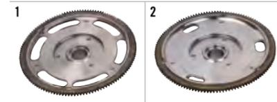
**1** In 1996 we started producing our own ultralight steel flywheels as all available flywheels at the time had certain problems. Harmonic balancer testing showed frequency problems at high rpm – from the flywheel. Our flywheel is more symmetrical and evenly balanced to be near perfect. The flywheel comes with the required distance pieces for mounting the straps.
