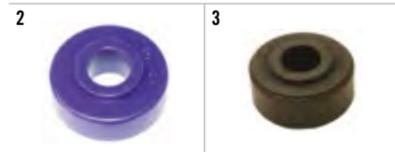
Mini Spares research program has encompassed the tie bar bushes. A well known fact amongst competition car drivers is that the outer bush needs to be hard to stop weaving when braking, increasing car stability.
