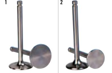
All our competition valves are produced in EN214N steel and require Manganese/ Silicon bronze alloy valve guides. They are stellite tipped and use the later narrow single collet groove unless stated and use current high efficiency valve head shapes and designs. The statutory use of unleaded fuel causes premature wear on valve stems therefore all our competition valves are heat treated to eradicate this problem.
