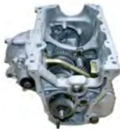
a. 4 Speed reconditioned A-plus rod change gearbox with 2.7 final drive [MSG27](#)
