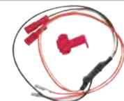
**Remote central locking upgrade for factory R/C Alarm.** By adding this alarm interface kit to the central locking kit (MSSK2001 / MSSK2004) you can operate the central locking using your existing Rover alarm remote control **MSSK2006**
