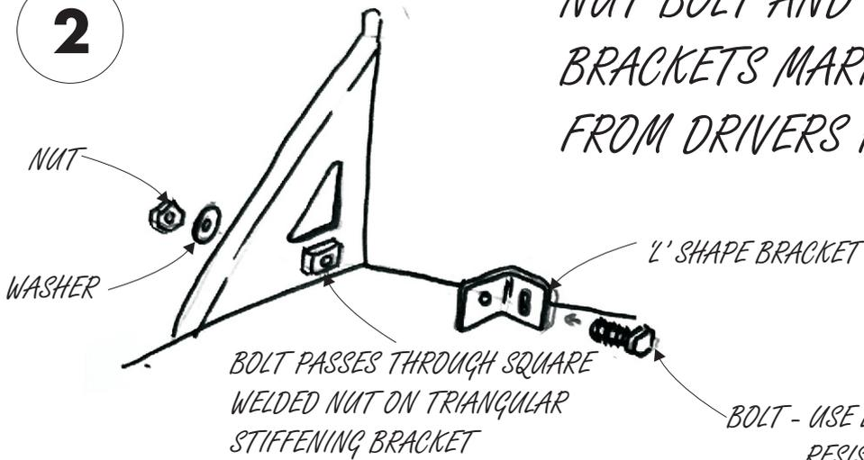
BOLT PASSES THROUGH SQUARE WELDED NUT ON TRIANGULAR STIFFENING BRACKET
