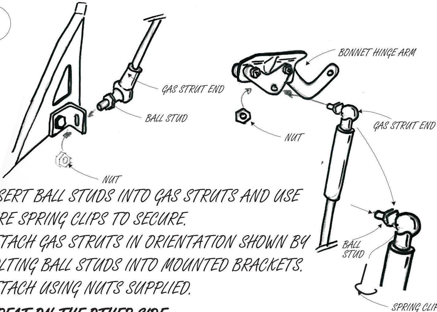
INSERT BALL STUDS INTO GAS STRUTS AND USE WIRE SPRING CLIPS TO SECURE. ATTACH GAS STRUTS IN ORIENTATION SHOWN BY BOLTING BALL STUDS INTO MOUNTED BRACKETS. ATTACH USING NUTS SUPPLIED.
