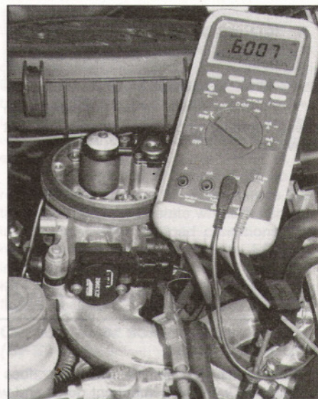
14.11 Check the throttle pot voltage output with the aid of a voltmeter
